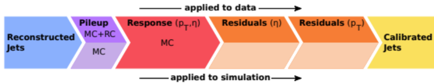
Figure 6.4: Graphical overview of the factorized approach used at CMS to apply jet energy corrections to data and simulated events.
