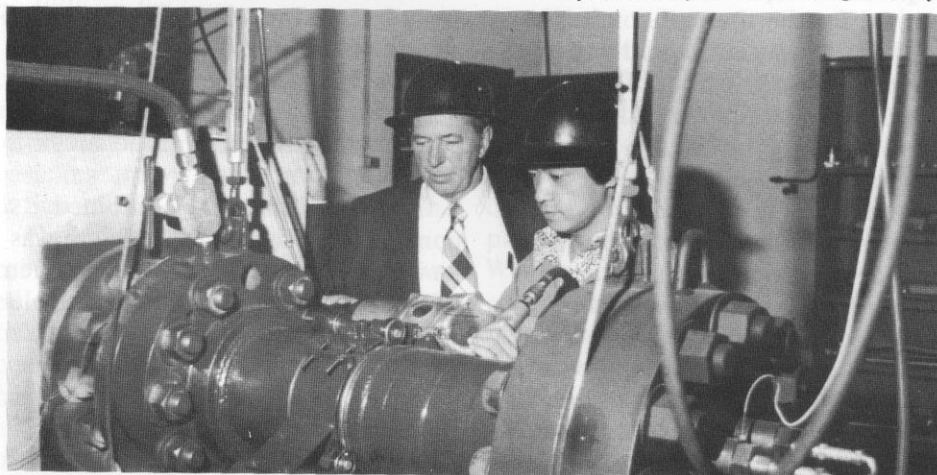
Professor Powell and Sang Kwak examine the cast concrete driver chamber. Hard hats are standard equipment when working with the forces of several hundred tons necessary to produce the shock waves.
