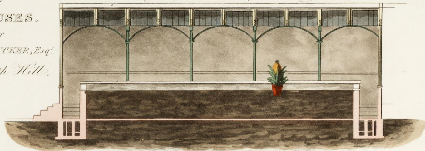
Longitudinal Section of one Pinery
