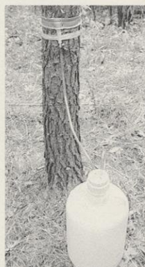
Stem flow collector. Water running down the tree trunk is captured and stored in the container for collection and analysis.
