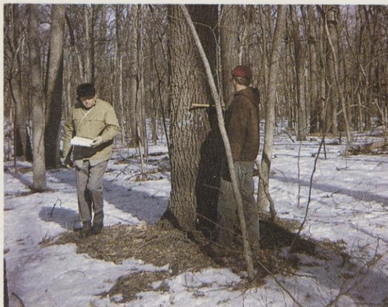
A Biltmore stick can measure diameter and tree height to give foresters an idea of volume.
