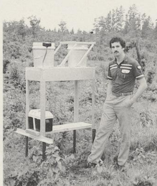
Wet/dry precipitation collector. One of the containers is for precipitation and the other for dry material, such as dust. The cover position is controlled by a sensor, which moves the cover over the dry material collector when it starts raining.
