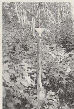
Forest water collector. Rain water is collected in the funnel, runs down the tube, and is stored in the container until collected for analysis.
