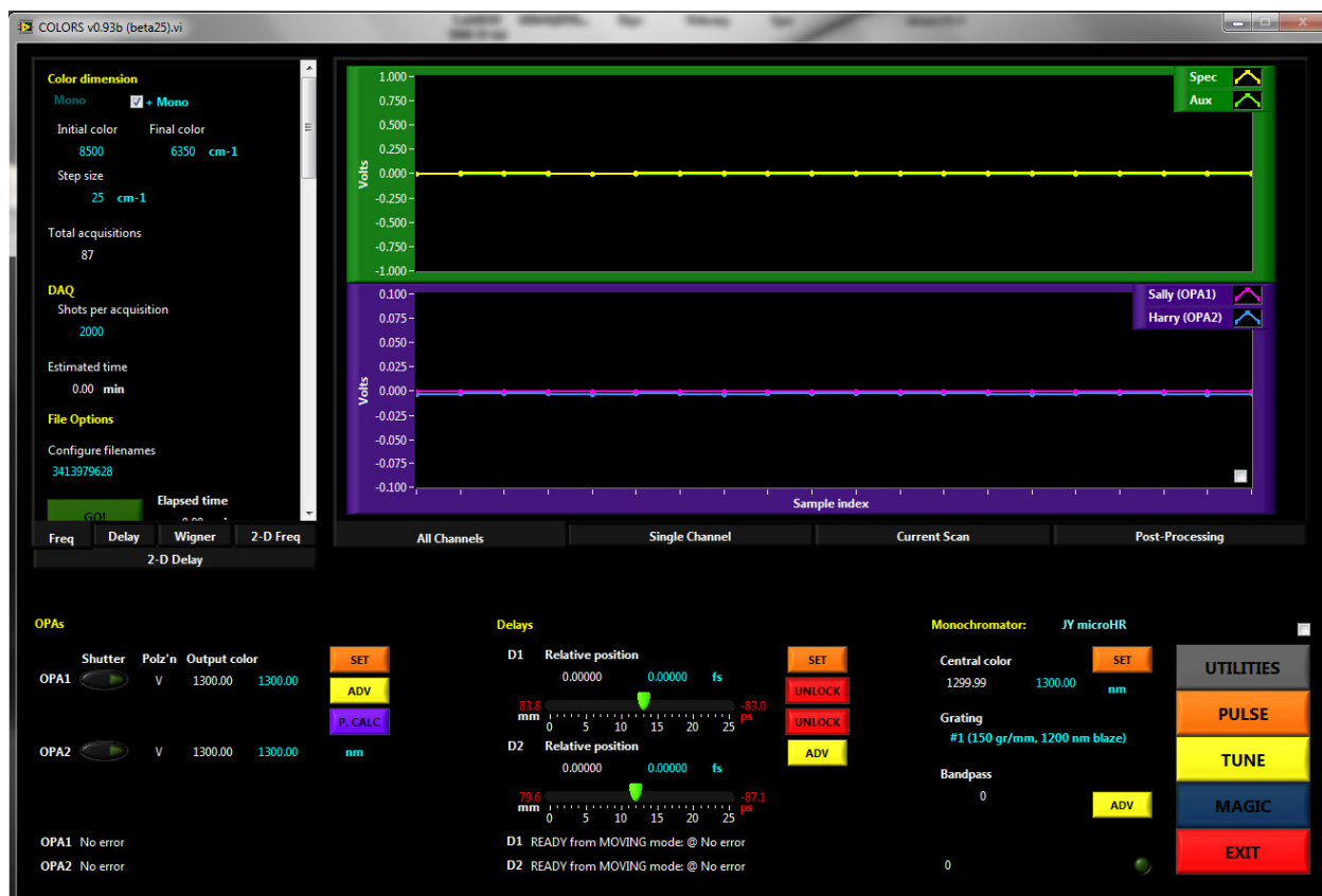
Figure D—COLORS main window. Scan parameters are set in the upper left corner. Simple OPA, monochromator, and delay controls are shown at the bottom of the window. ColorTune and PulseScan modules are accessed by the TUNE and PULSE buttons in the lower right corner. An active report of voltages for various channels is shown across the top. The tabs below this voltage screen also provide the option of watching the scan in progress (“Current Scan”) or plotting and processing existing data (“Post Processing”).
