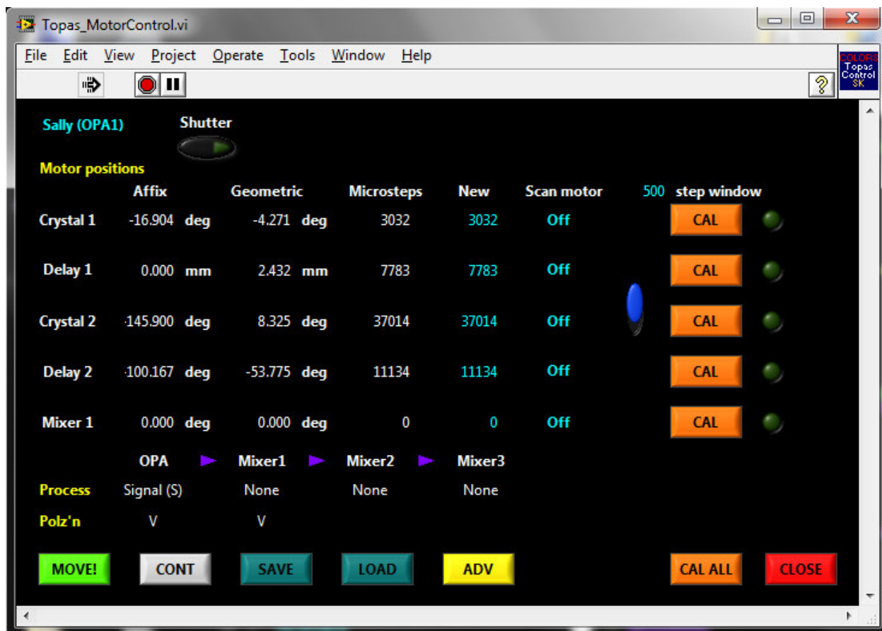
Figure 4—Topas “Advanced” controls. Common uses in alignment are described in the main text. To manually change an actuator, enter the desired microstep value in the appropriate row of the “New” column and press the “MOVE!” button. Alternatively, press the “CONT” button for continuous reading of the “New” column and either enter the desired new position or place the cursor after any digit in the existing entry and use the up and down arrows on the keyboard to change the values. In each case, the change will have taken place by the time the value shown in the “Microsteps” updates. The “Geometric” column is the physical position or angle of the corresponding OPA element. The “Affix” is a static offset. The geometric angle is calculated by multiplying the Microsteps value and a conversion constant, then adding the affix.
