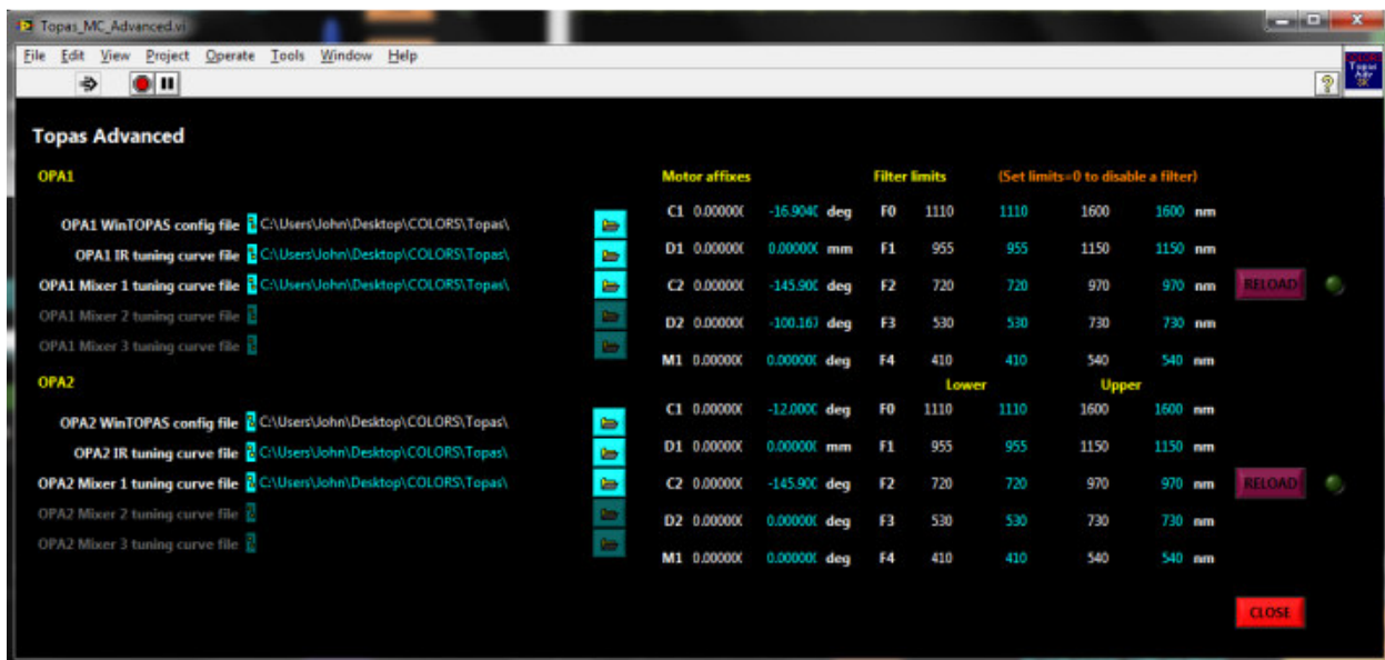
Figure 5—Topas Advanced Advanced window. When adjusting tuning curve files, this window can be used to reload the curves into LabVIEW. Simply press the appropriate RELOAD button. If the file path still appears on the left-hand side of this window, then the reload was successful.
