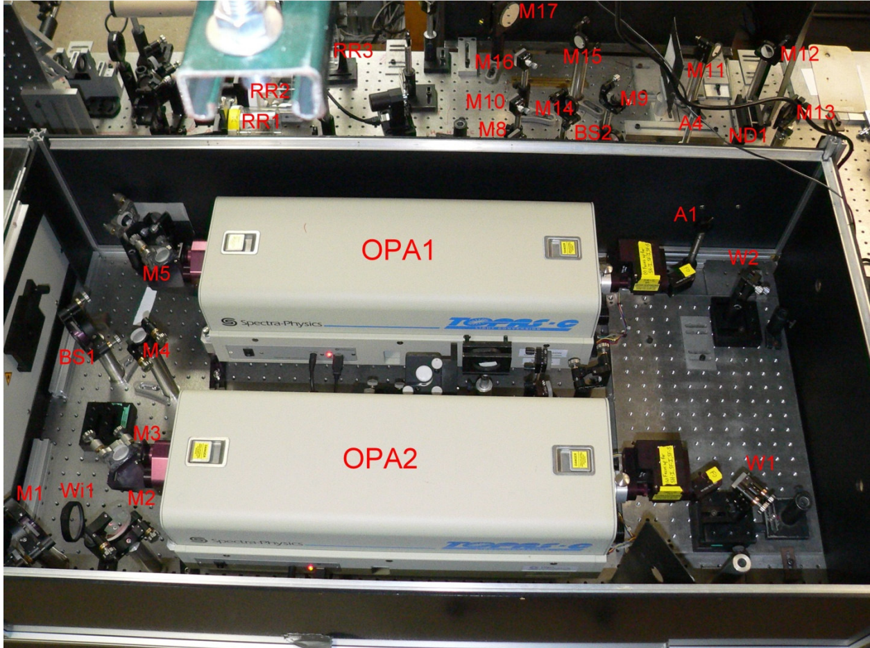
Figure C1— Optical table near the OPAs with element labels. The figure shows the area after the OPA area enclosure was completed and the chirp compensation window (Wi1) was placed before OPA2.
