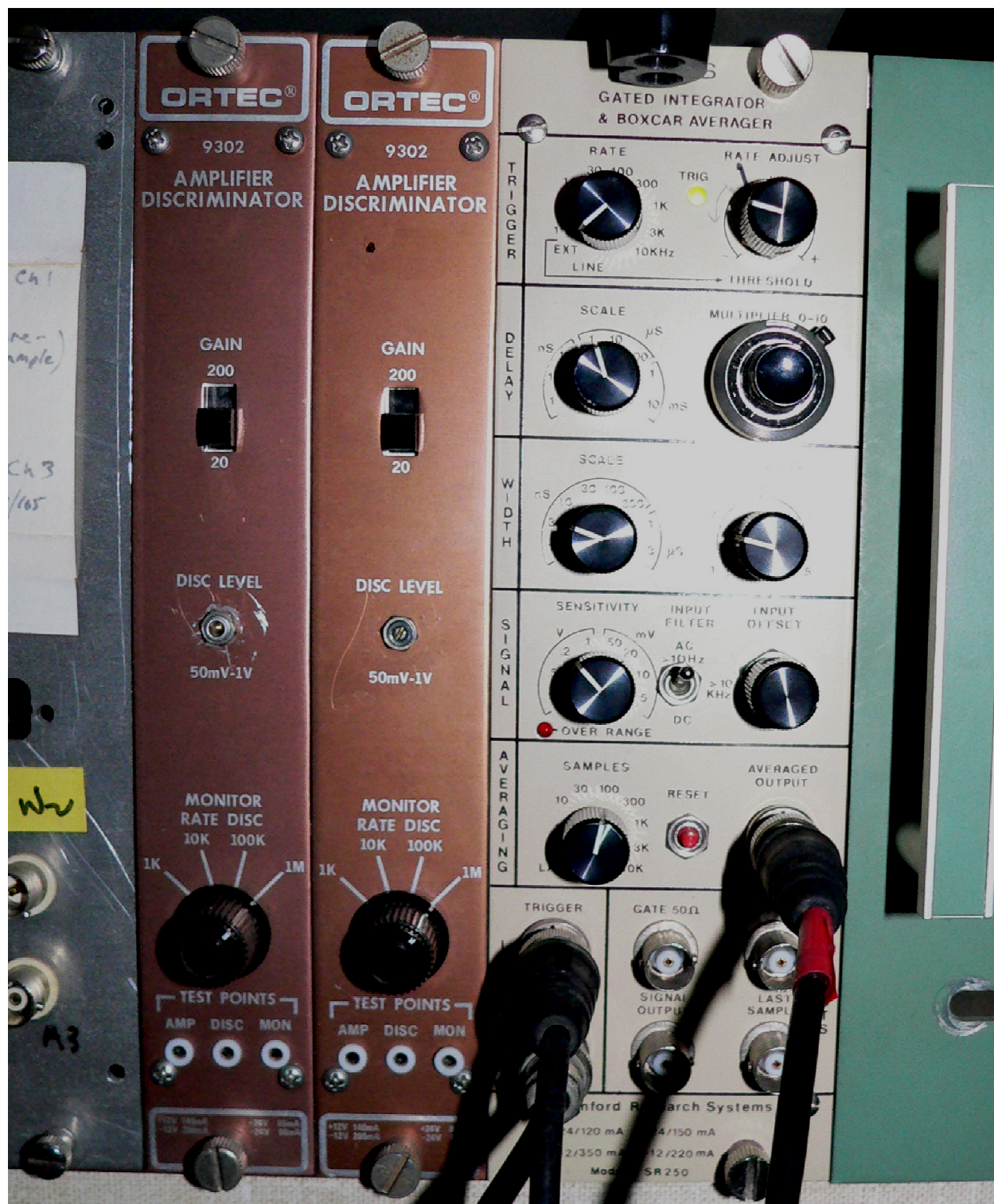
Figure 8—Boxcar averager. Notice in particular the output cable (shown with red tape) connected to the “AVERAGED OUTPUT” BNC, used when active background subtraction
