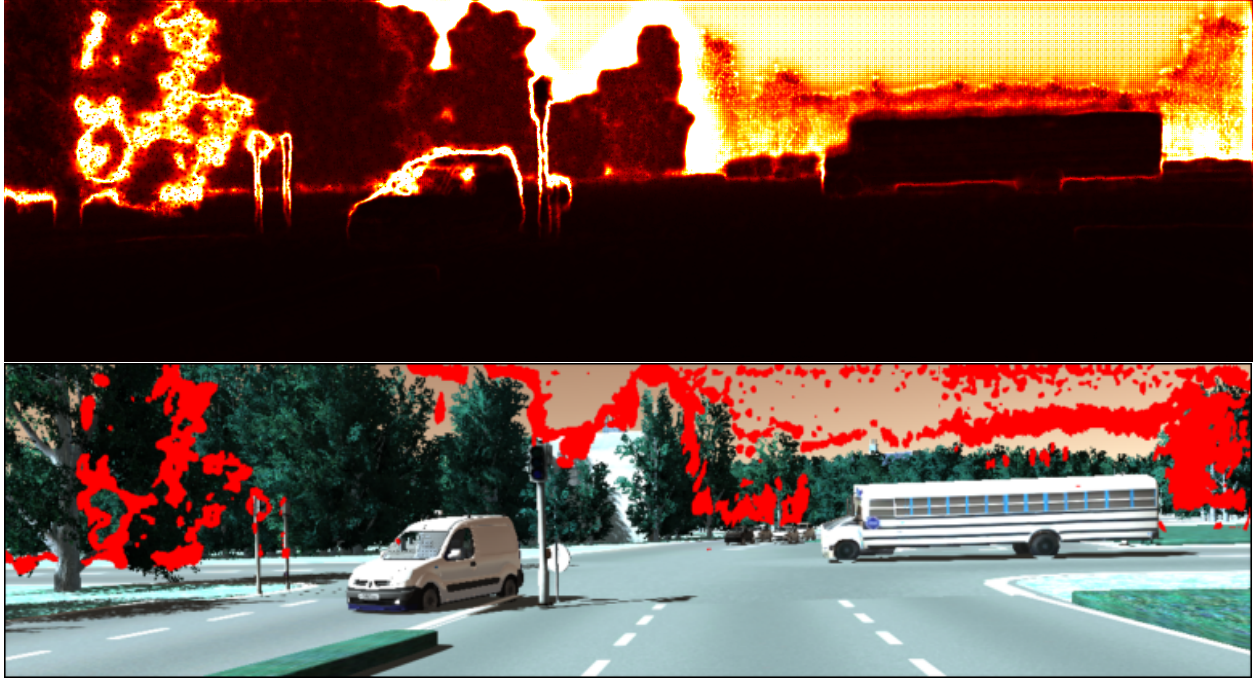
Figure 4.1: Top is a raw uncertainty of the depth estimation process. Bottom is significant region selected by our method, with theoretical guarantees to restrict family-wise error rate. This region can be used for calibration by practitioners.
