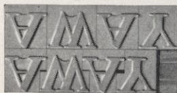
TYPE "BEFORE AND AFTER" MATCHING ON THE ROUSE TYPE MORTISER. NOTE PERFECT SPACING AND EXACT JUSTIFICATION.
