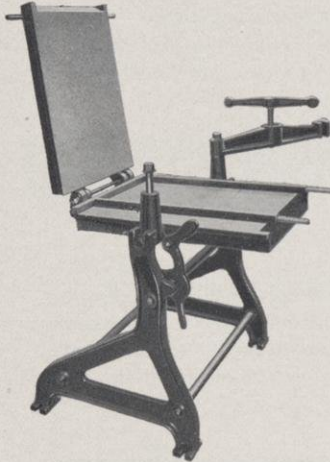
SUPERIOR CASTING BOX, OPEN, WITH BEARER GAUGES
