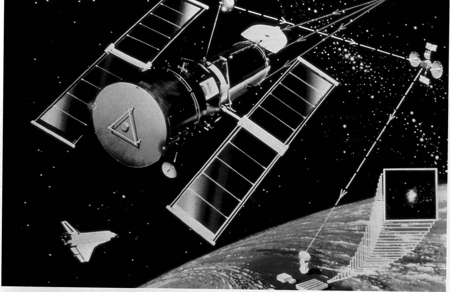
Here the HST is shown in orbit receiving light from a distant star. The telescope's mirror directs the light to various onboard instruments that process and record data, then transmit it to a Tracking and Data Relay Satellite (at right). In turn, the data is sent to earth stations at White Sands, New Mexico, and to NASA's Goddard Space Flight Center outside Washington.
