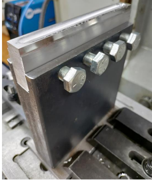
Figure 45: Image of the custom workpiece fixture used for samples that will be imaged via the X-ray beamline
