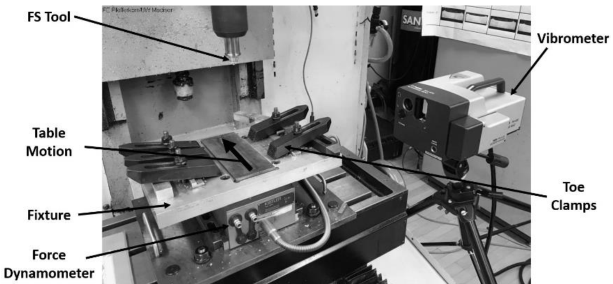
Figure 18: Image of the experimental setup consisting of the laser vibrometer in relation to the force dynamometer and workpiece clamping system
