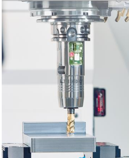
Figure 47: Image of Schunk iTENDO toolholder being used during a milling application (Taken From: https://schunk.com/at_en/homepage/itendo/ )
