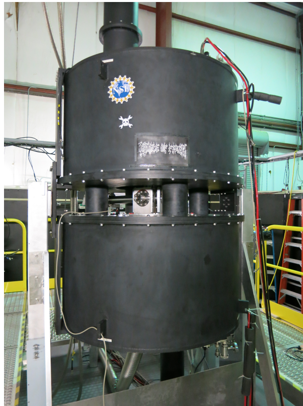
FIGURE 4.6: Picture of the super conducting magnets of MDPX in black. The two sets of magnets are separated by a large air gap housing the UHV chamber used for this study.
