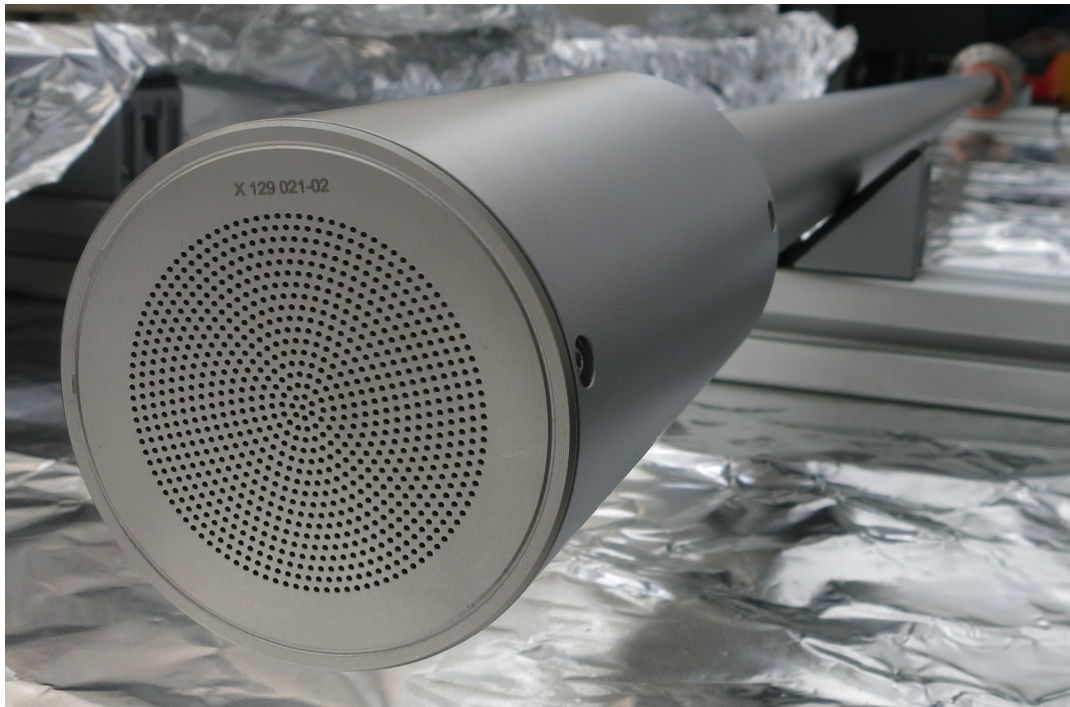
FIGURE 4.18: Picture of a the hole diaphragm on the front plate of the probe head space
