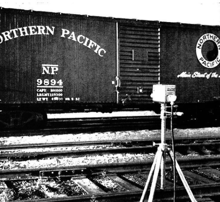
A lightweight TV camera, stationed in a yard of the Baltimore and Ohio Railroad, observes car numbers in a unique demonstration
