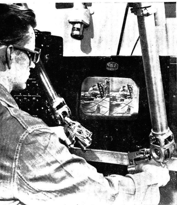
At Argonne National Laboratory, "stereo" or three-dimensional television enables men working with radioactive substances to view them safely
