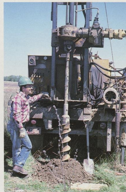
Wells are the "eyes" of groundwater researchers. Mike Lembcke of the Wisconsin Geological and Natural History Survey pierces the soil with a drilling rig; the new well will reveal another drop of knowledge about groundwater.
