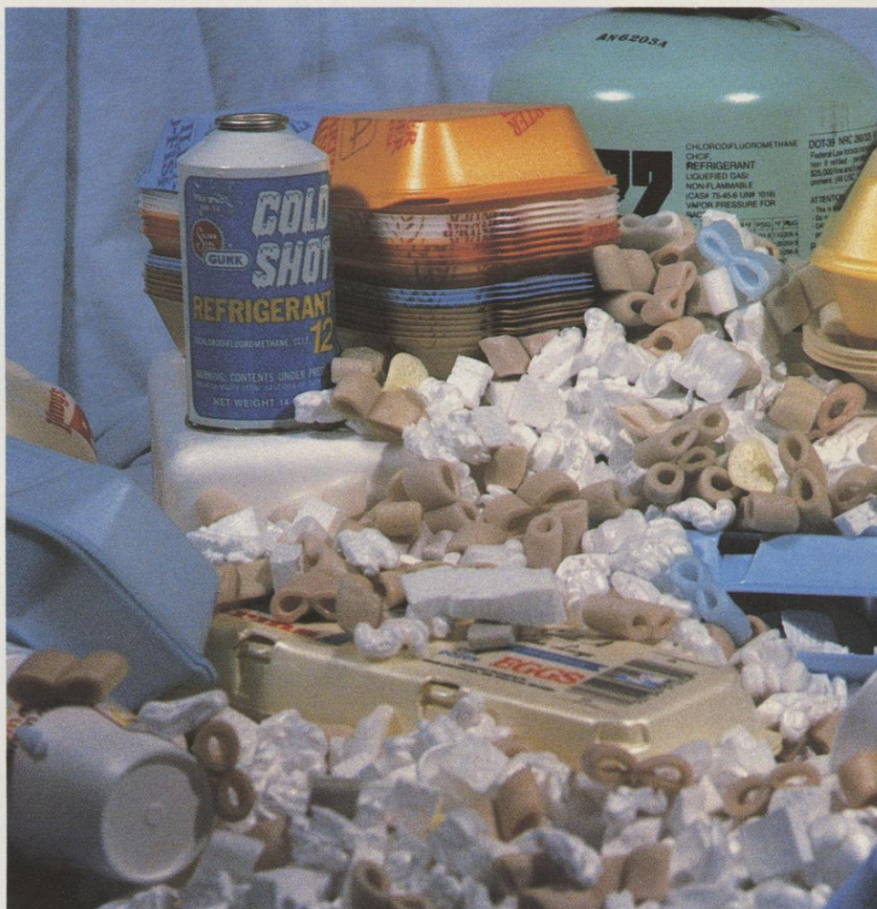
Injected into molten plastic, CFCs bubble up a foam, then are released into the atmosphere as waste. The foam is formed into fast food containers, cups, packaging material and other products. Photo by Bob Queen
