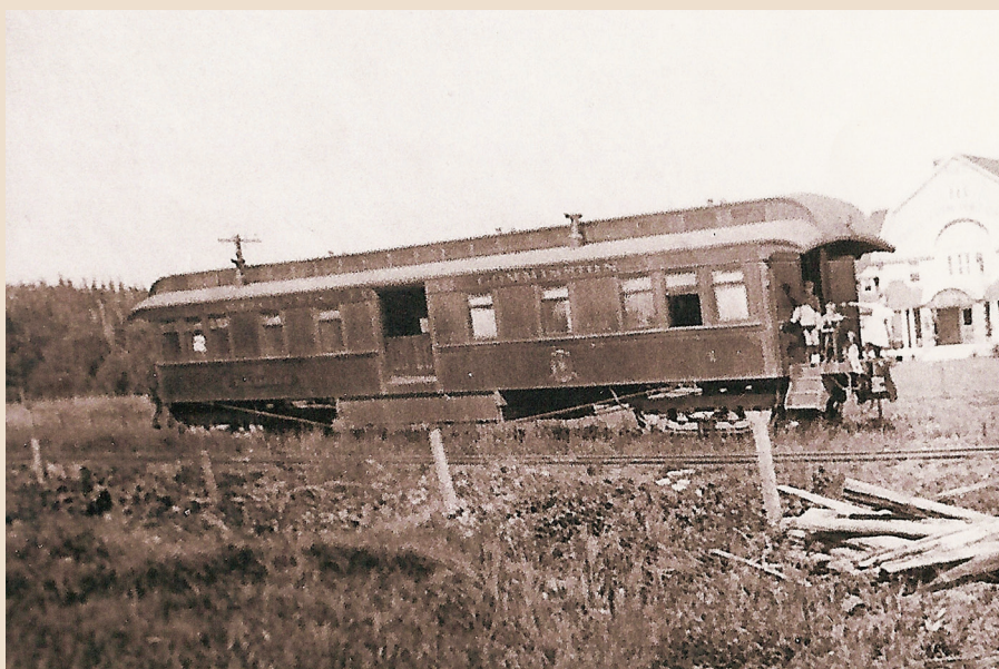
The Badger railcar in front of the 1897 hatchery building. The car contained aerated tanks to transport fish to stocking locations.
