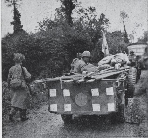
HOME-MADE AMBULANCE. A jeep with racks built to carry stretchers takes a wounded man to the rear.
