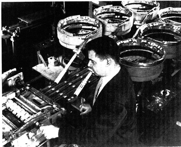
A machine in which conducting circuits are automatically printed on ceramic wafers. This is part of an experimental automatic production process in which electronic components are built up with these basic wafer units.
