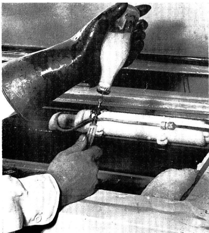
The progress of the bottle polymerization is followed by periodically withdrawing a sample in a small syringe and determining the amount of rubber in the withdrawn sample.
