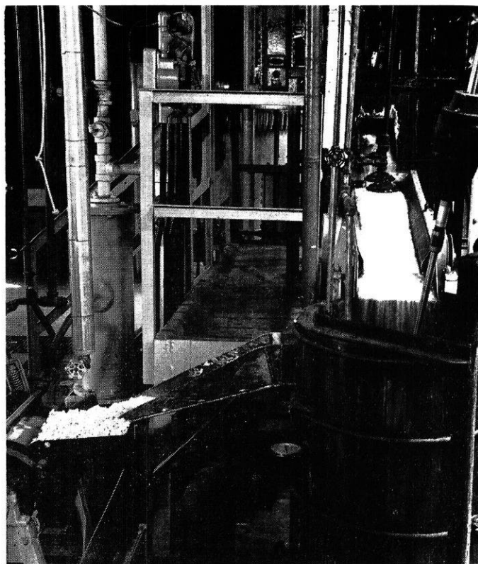
Latex from the blend tank is coagulated in the continuous operation as pictured. Rubber crumbs formed in the upper tank spill onto a screen which separates the fluid. The crumbs are washed by water sprays and tumble into the "soap conversion" tank below where any remaining soap is converted into fatty acid. The crumbs then tumble onto the rotary filter at lower left where the excess water is squeezed out.
