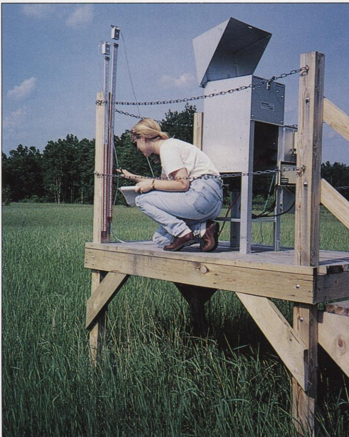
Air monitoring stations will continuously measure air quality in the area to make sure the mine meets all air standards.
