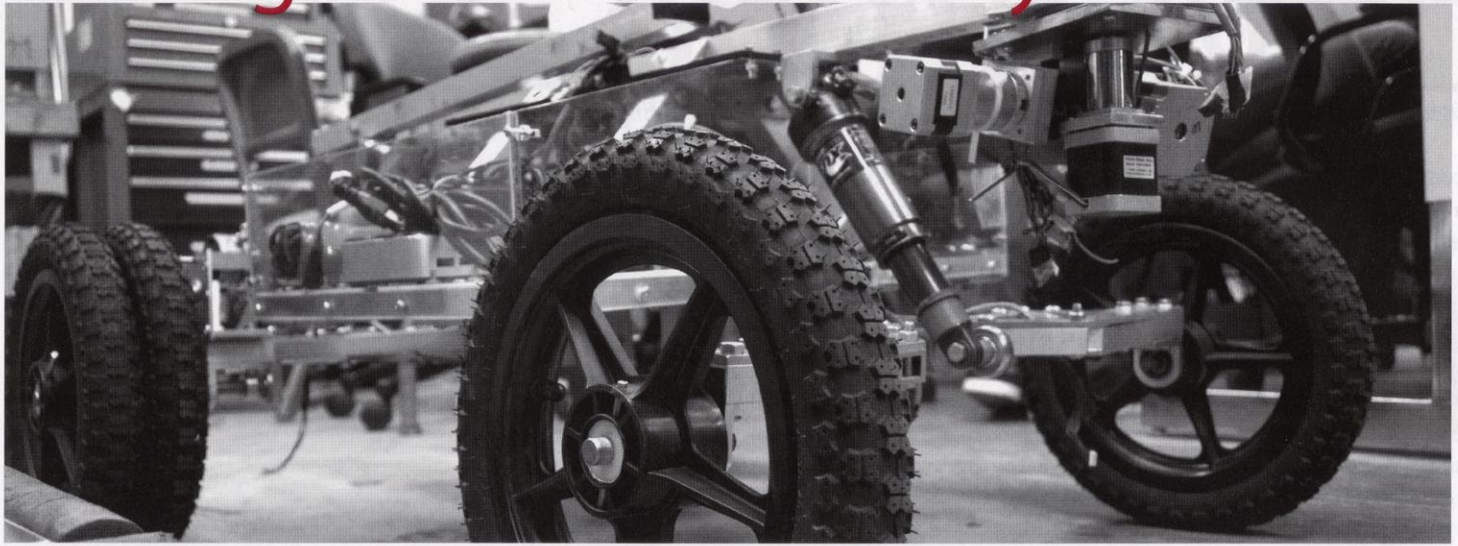
Scorpio is Wisconsin Robotics' RASC-AL competition robot and was designed to remotely traverse difficult terrain and pick up specifically colored rocks.
