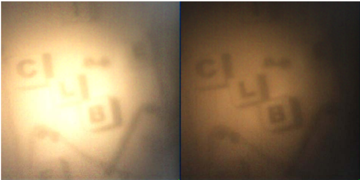
Figure 4.13 Reduction in glare with the use of a polarizer as seen from comparison of an image without using a polarizer in front of a tunable camera (left) and the same image captured with a polarizer in front of the lens (right).
