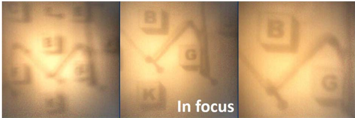
Figure 4.14 Images of a test scene as captured by a single camera while the focal length of its tunable liquid lens was being tuned using a microheater.
