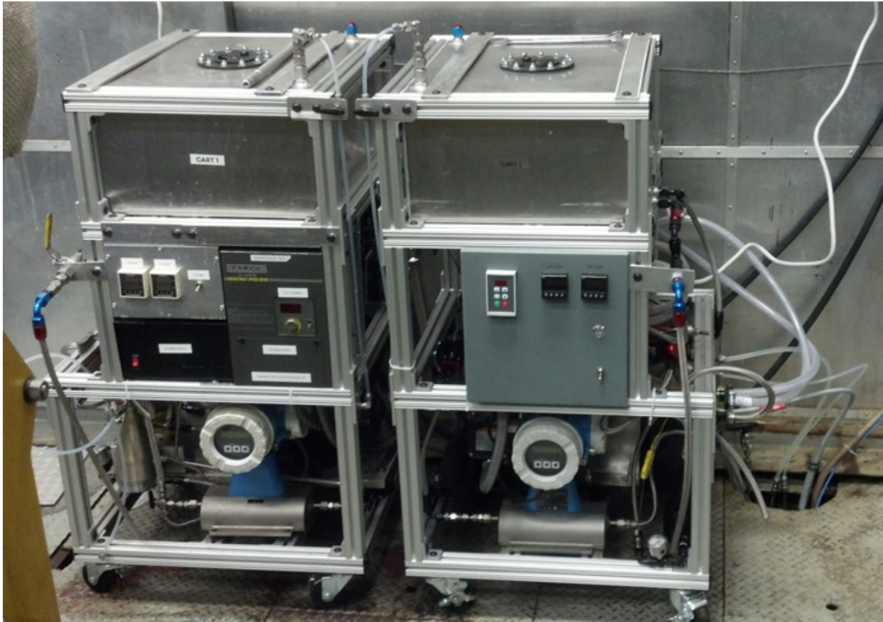
Figure 3.4: Picture of the two liquid fuel carts, with the common rail Cart 1 on the left and the port fuel Cart 2 on the right.
