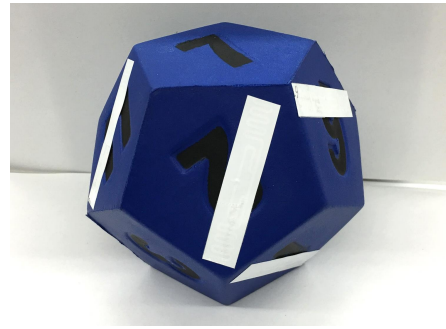
Figure 2.33: Eight tags are attached to the surface of a 12-side dice.
