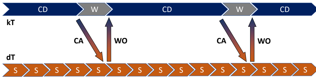
Figure 2.1: Ideal collaboration pattern, where the dynamic thread advances the physics continuously while the kinematic thread occasionally waits for a work order.
