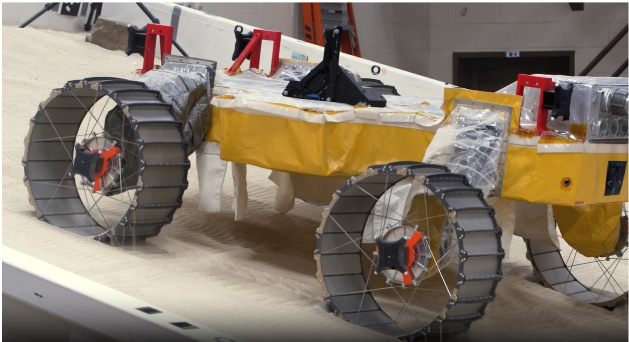
Figure 3.12: MGRU3 climbing a “tilt bed” in NASA’s SLOPE lab testing facility.
