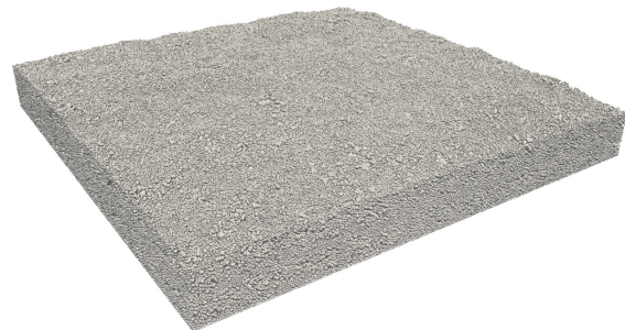
(f) The final settled and compressed base DS patch.
