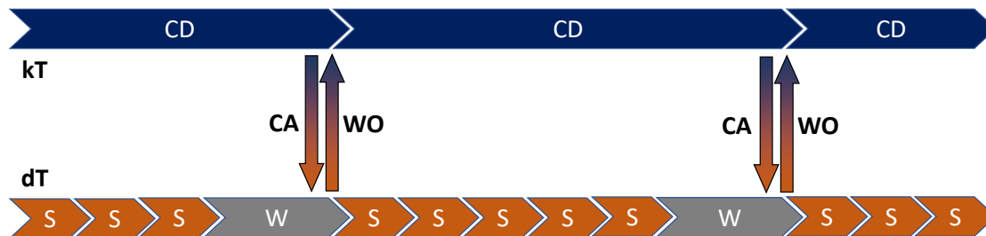
Figure 2.2: Unideal collaboration pattern, where the dynamic thread advances waits for the kinematic thread occasionally to generate the contact array. DEM-Engine will automatically avoid this scenario.
