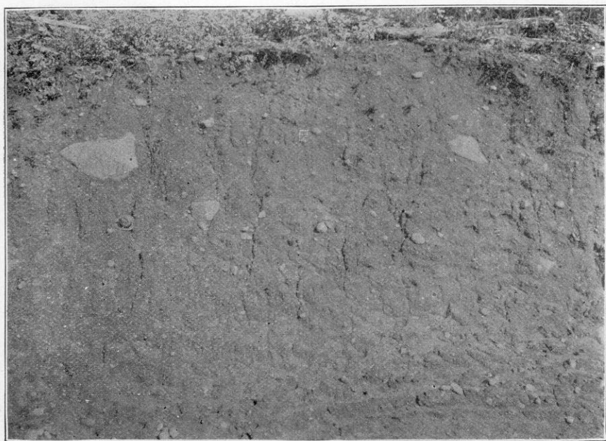
FIG. 2. SECTION OF CHELSEA CLAY LOAM. TYPE OF GLACIAL SOIL. Four miles east of Antigo, Langlade County. Shows fifteen feet of surface and subsoil consisting of sandy clay mixed with boulders.
