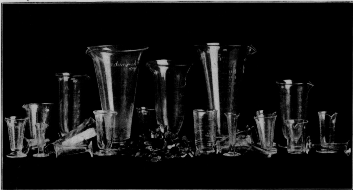
Fig. 19. —Prescription Graduates and Weights. There are over 700 apothecary and metric weights in the pile in the center of the picture, many of which were from 3% to 10% light. Some of the glass graduates are 15% too large, made this way by careless manufacturers. These weights and graduates were used by druggists in prescription work.
