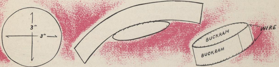
(a) Cut and wire 3\frac{1}{2} " circle of buckram. (b) Sew 2" strip of buckram to same wire. (c) Wire bottom of tip after ends are joined.
