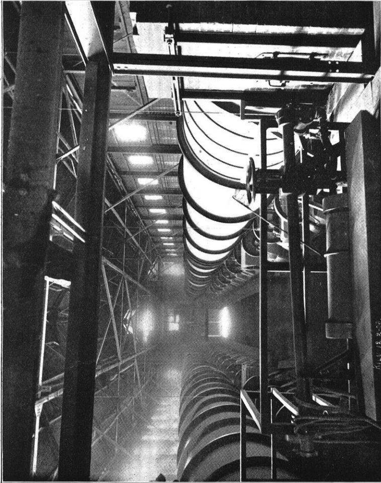
Rotary Kilns, 150 feet long, Edison Cement Co., Steubenville, N. J.
