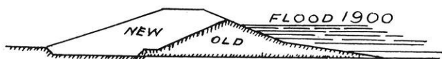
Fig. 7—Cross Section of the United States Levee and the Proposed New Addition to It.
