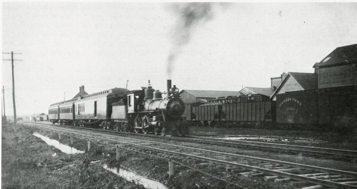
Locomotive No. 20, a 4-4-0 American Type, is pictured heading east through Ladysmith with either No. 8 or No. 84. Note the roof and two chimneys of the Soo Line depot (built in 1904) above the coaches.
