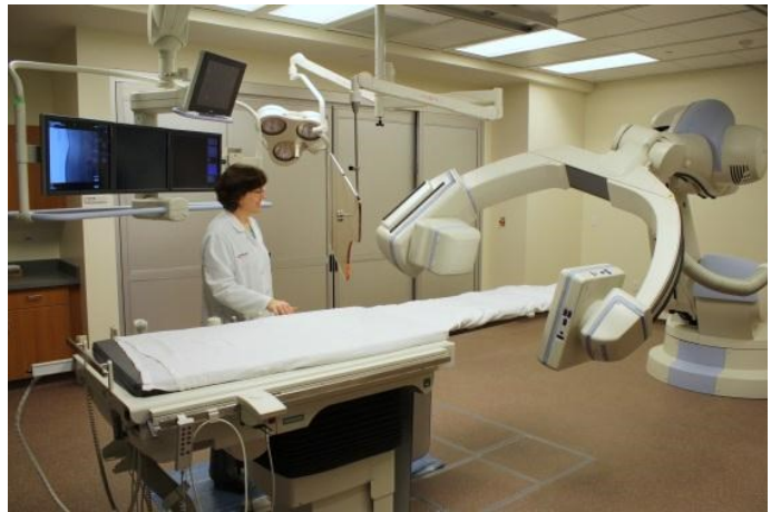
Figure 1-1: Robotic C-arm based angiographic imaging system (Artis zeego, Siemens AG, Forchheim Germany)
