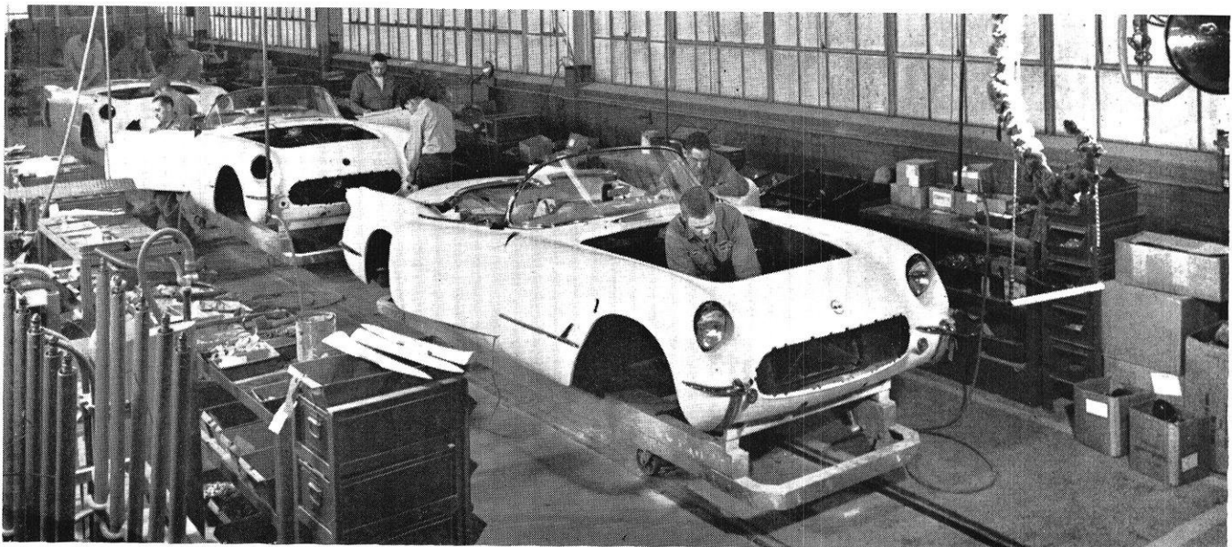
Here the completed fiberglass body moves down the trim assembly line.
