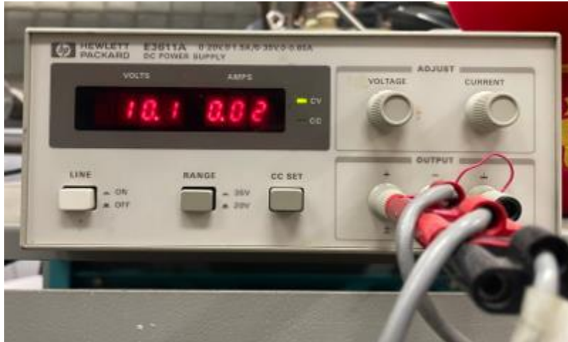
Figure 3-14 The HP3611A power supply supplies the 10-V constant voltage to the Endevco pressure transducers.
