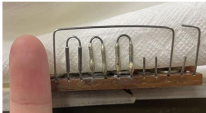
Figure 3-7 The fabrication of the leftmost U-bend for the 5-turn PHP
