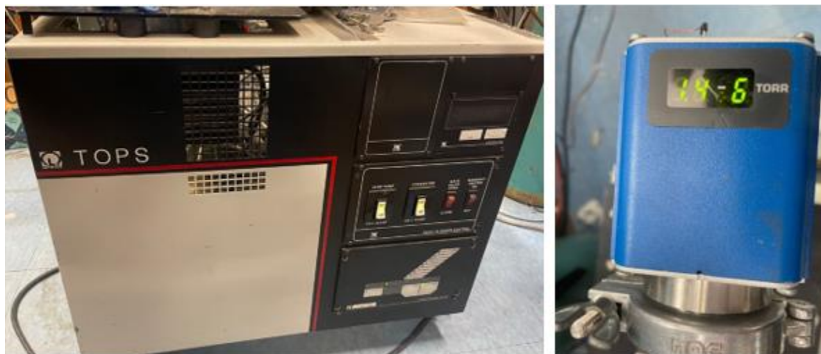
Figure 4-4 Mechanical/turbo pump station for evacuating the gas line and the vacuum chamber and the of the vacuum Dewar pressure is at 1.4 \times 10^{-6} Torr ion-gauge during the experiment.
