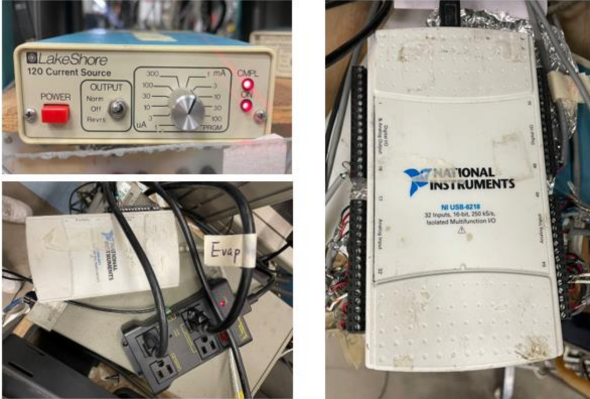
Figure 3-13 The LakeShore 120 Current Source supplies the current of the PRT temperature sensors (top left). NI USB-6211 and the relay (lower left) will shut down the power supply of the heaters in case of power shortage, water pump failure and other accidents. NI USB-6218 (right) measures the voltage across the temperature sensors and the voltage from the pressure transducers.
