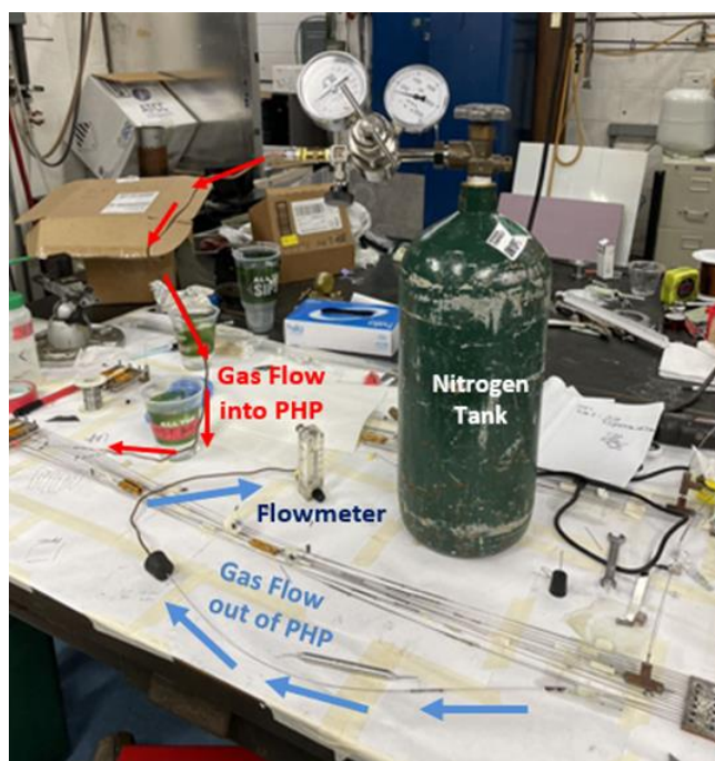
Figure 4-1 The PHP1 is checked for the clogging before closing the last joint of the capillary tube on the adiabatic section.
