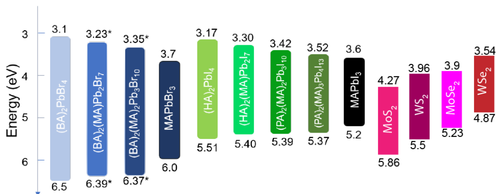
Figure 1.9 Band diagrams of 3D halide perovskite, 2D RP halide perovskite with different n number and TMDs.
