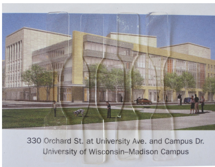
Figure 3.2 Transparency (from left to right) of neat PVOH and PVOH/NFC nanocomposites with 2.5%, 5%, and 10% NFC, respectively.
