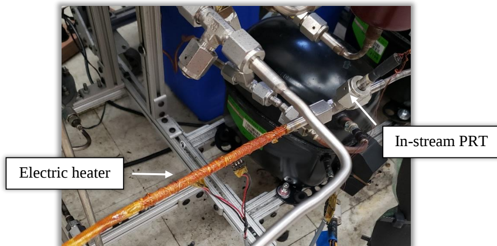
Figure 5.17. Photo of the electric heater and in-stream PRT before first compressor.
