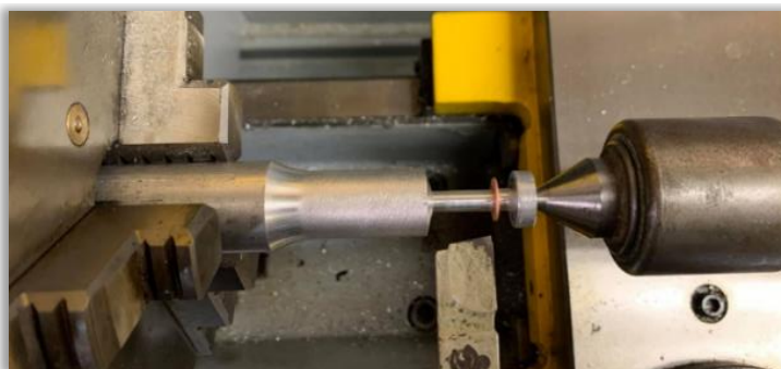
Figure 8.18. Machining set-up to turn down pre-made JT orifices.
