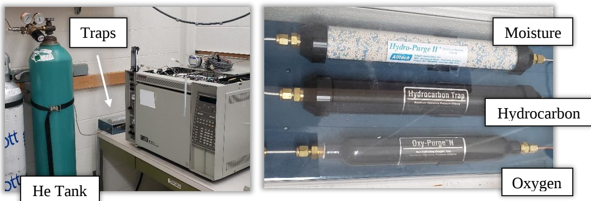
Figure 5.38. Photos of moisture, hydrocarbon and oxygen traps.
