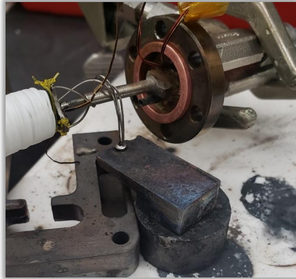
Figure 6.8. Soldering of heat exchanger tubing to sleeve.
