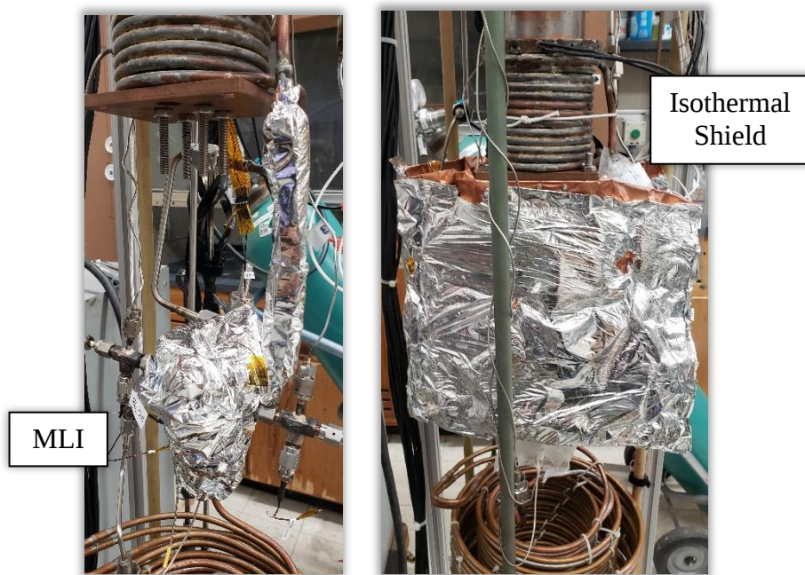
Figure 5.32. Photo of MLI and isothermal shield.
