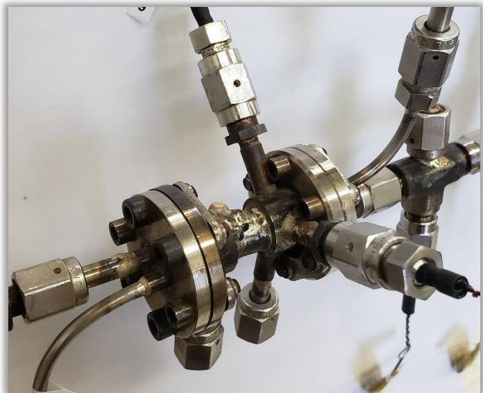
Figure 5.13. Fully assembled test section.
