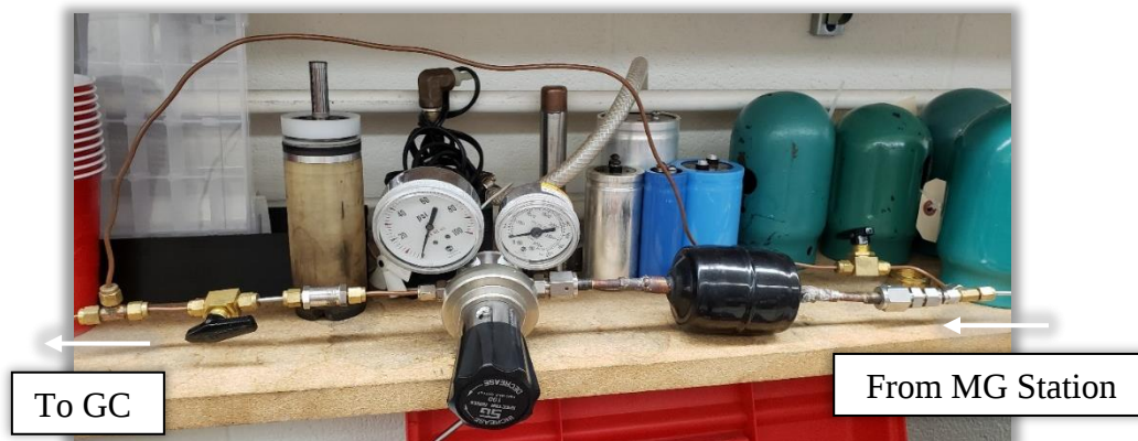
Figure 5.39. Photo of mixed gas sampling line to the GC.
