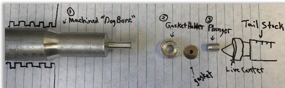
Figure 8.18. Machined tools for turning down pre-made JT orifices.
