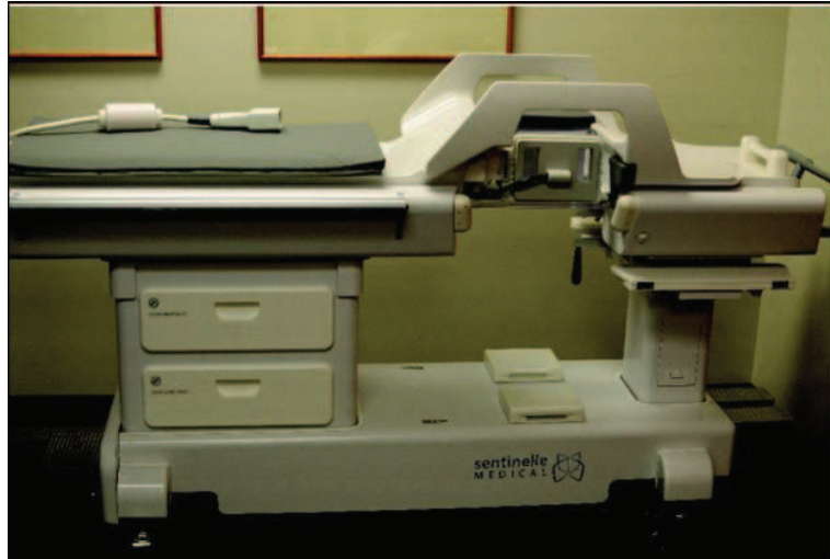
Figure 2.1 Photograph of the patient support platform of a commercial breast MRI system.
