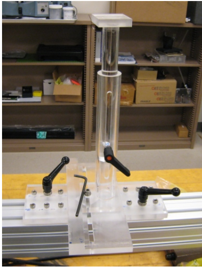
Figure 3.2: The constructed source holder for the CDS with the platform holder.
