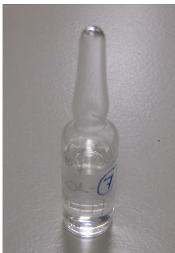
Figure 4.1: Photograph of the ^{90}\text{YCl}_3 radioactivity standard solution from the NIST SRM program in a flame-sealed ampoule.
