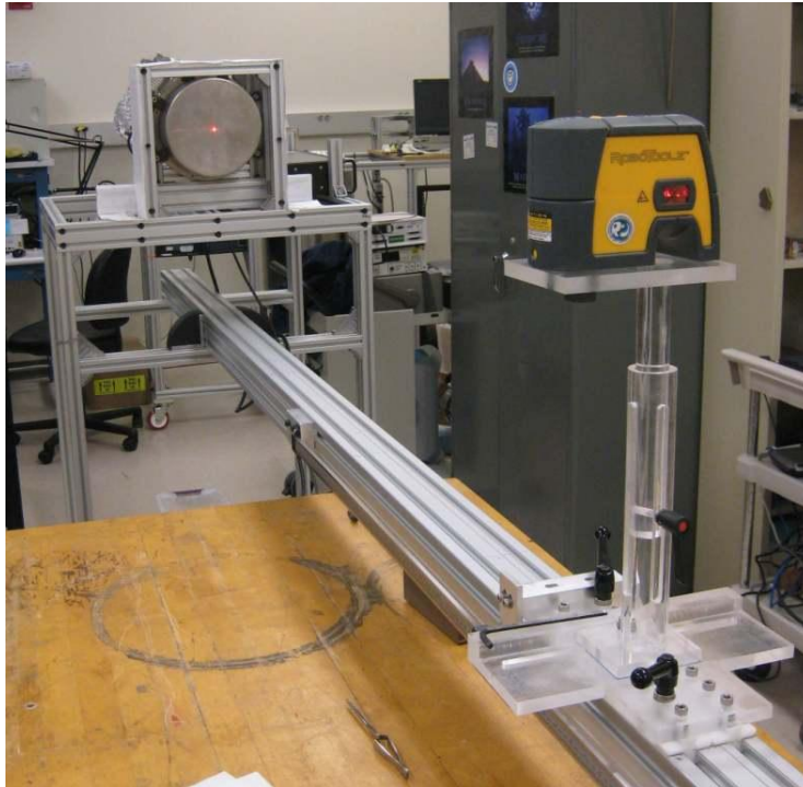
Figure 3.3: The Robotoolz self-leveling laser (in source holder mount) used to position the detectors.
