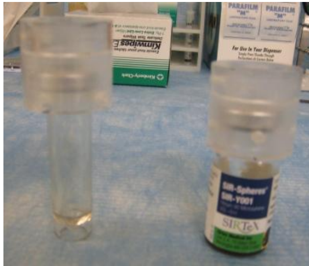
Figure 5.3: Photograph of the source holder collars attached to the v-vial (left) and the shipping vial (right).
