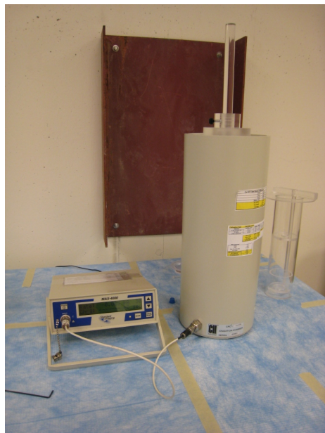
Figure 5.2: Photograph of the Capintec 12 atm dose calibrator connected to a Standard Imaging Max 4000 electrometer.
