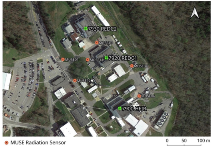
Figure 3.1: MINOS radiation sensor network distributed around HFIR and REDC, labeled. There are six radiation detectors in total (red), placed along roads used as routes for material transfers. (Image source: [28])
