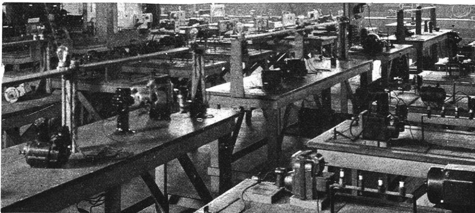
General view of the Starting and Lighting Laboratory at the S. of E. Every table contains a complete starting, lighting, and ignition system of some make of car, each one laid out exactly and complete as it is in the actual car.
