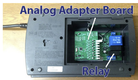
Figure 3.5: The internals of an Emonix smart power strip include a relay to switch power to the plugs it serves and an analog adapter board to sense the power consumption of the connected appliances. The main CPU sits beneath the analog adapter board along with its WiFi interface that directly connects to the home’s network. This allows energy measurements to be relayed to an off-site controller.
