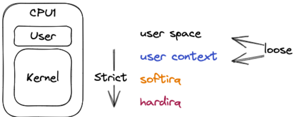
Figure 4.1: Lower level context (closer to hardware) has higher priority. Userspace and usercontext can preempt each other.
