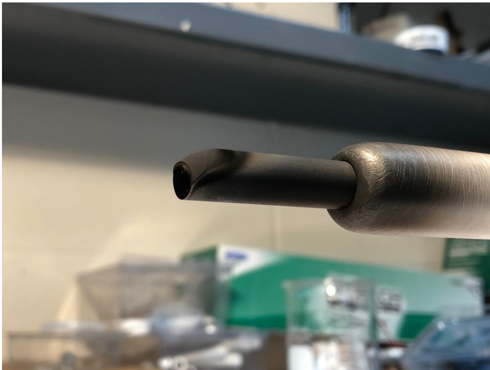
Figure 4.10.: 1 cm diameter, 3.3 cm long solid graphite tip of an insertable probe used to increase carbon levels in the machine. Deformation in the tip of the graphite is due to plasma exposure after two run days with 500 kA QSH plasmas.
