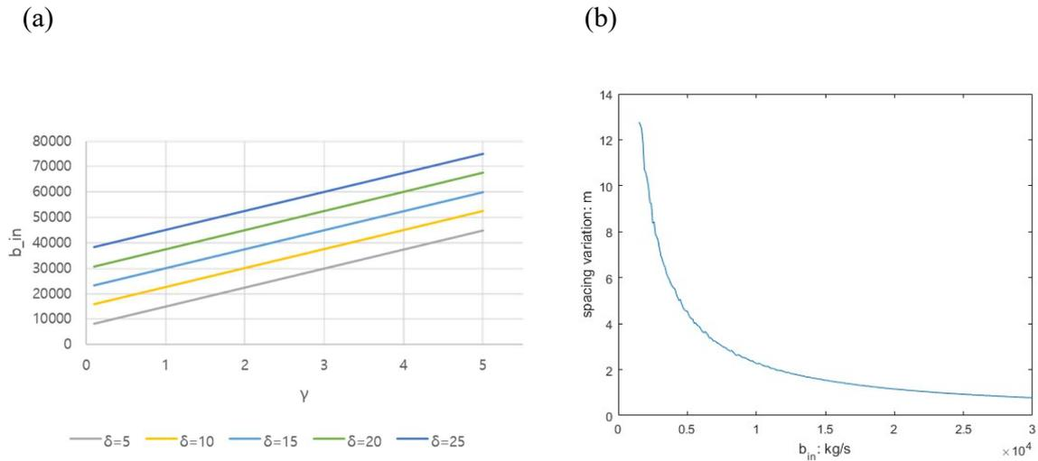
**FIGURE 5.6** Sensitivity analysis for  $b_{in}$  (a)  $b_{in}$  versus  $\gamma$  and  $\delta$ ; (b) spacing variation versus  $b_{in}$
