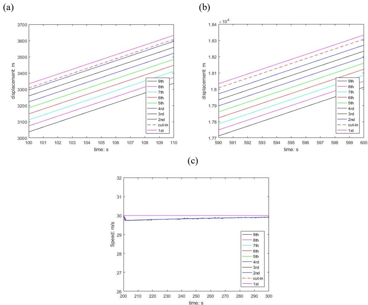
**FIGURE 5.9** Spacing increment for cut-in (a) trajectory at the start; (b) trajectory of attaining spacing for cut-in; (c) speed profile
