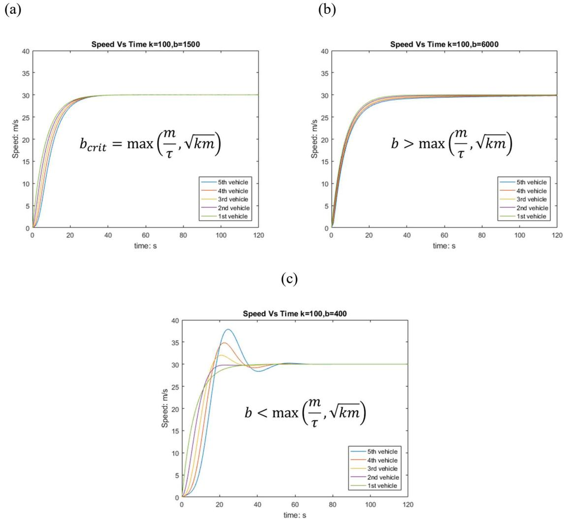
**FIGURE 3.3 Types of damping (a) Critical-damping; (b) Over-damping; (c) Under-damping**
