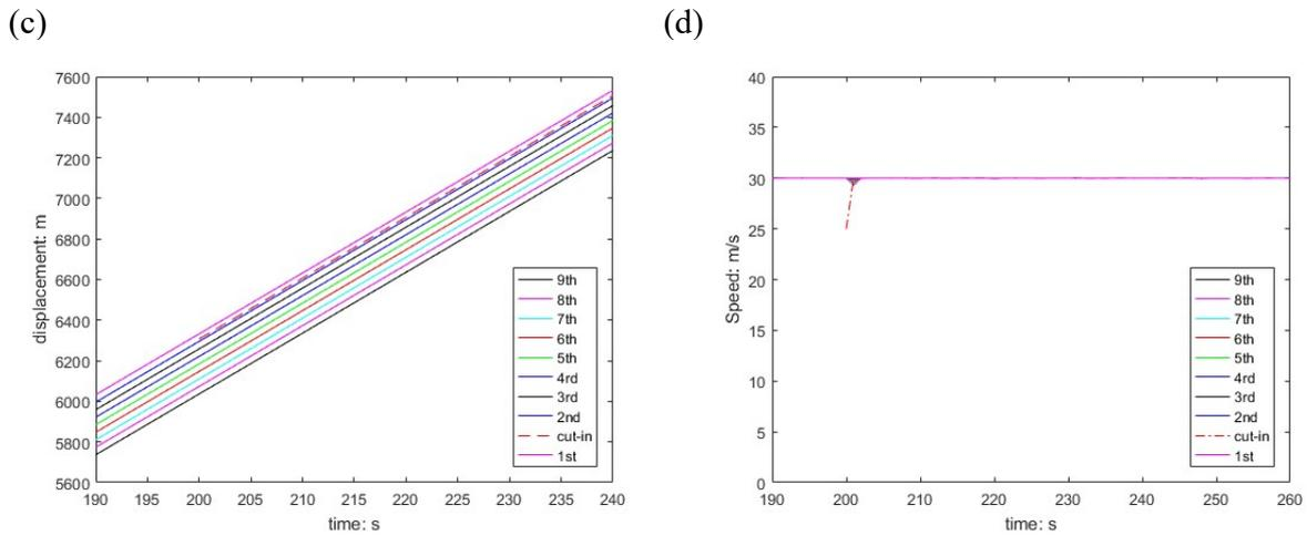
**FIGURE 5.8 Trajectories and speed profiles of the case of merging from on-ramp to mainline (a) Trajectory of no control; (b) Speed profile of no control; (c) Trajectory of control; (d) Speed profile of control**
