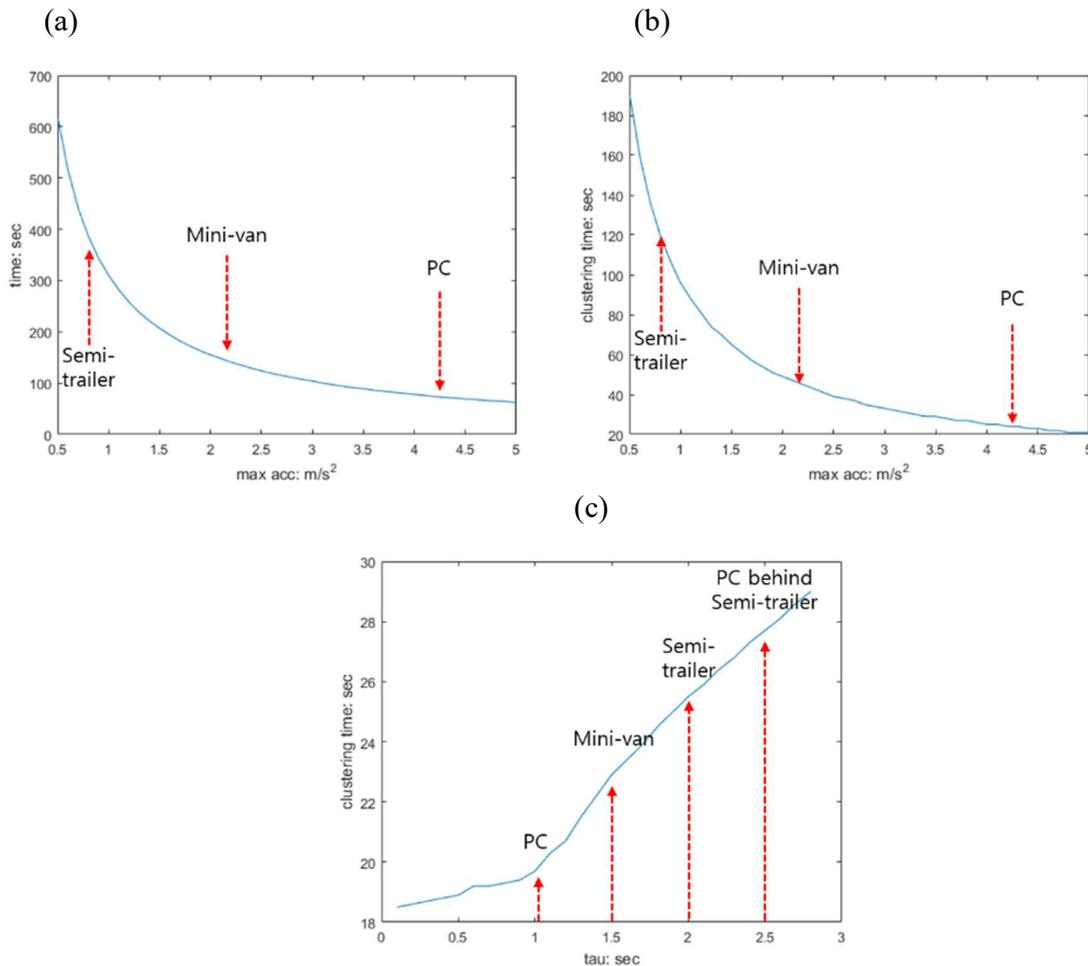
**FIGURE 6.1** The effect of  $a_{max}$  and  $\tau$  (a) the time that reach  $v_d$  vs.  $a_{max}$ ; (b) Clustering time vs.  $a_{max}$ ; (c) Clustering time vs.  $\tau$
