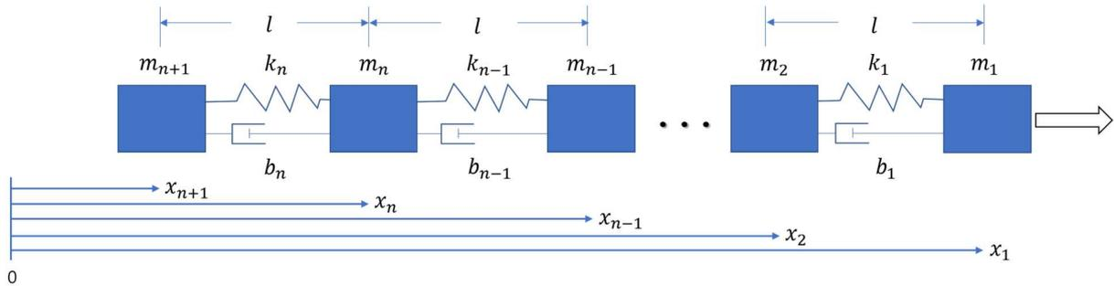
**FIGURE 3.2**  $n$  body  $n-1$  spring and damper system
