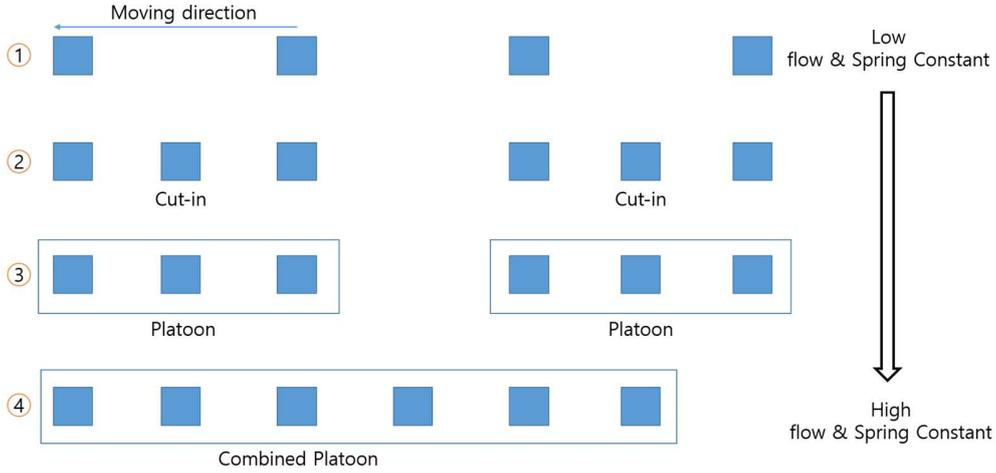
**FIGURE 4.1 Evolution of vehicle platooning**
