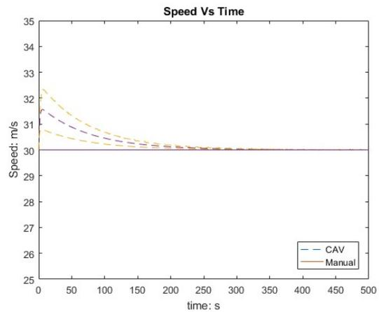
**FIGURE 7.4 Platooning procedure in mixed traffic (50% proportion of Manual vehicle)**
