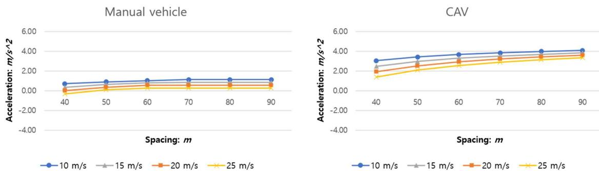
**FIGURE 7.2 Comparison of acceleration between a manual vehicle and CAV**
