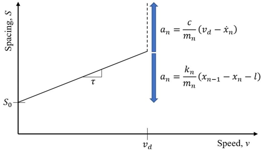
**FIGURE 7.1 Relationship between spacing and speed in Newell's model**
