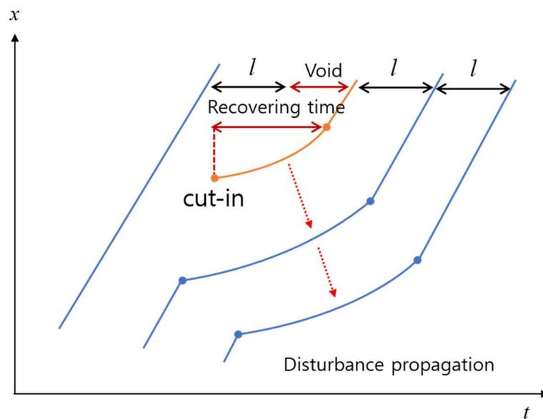
**FIGURE 5.2** Occurring void resulted from a cut-in vehicle
