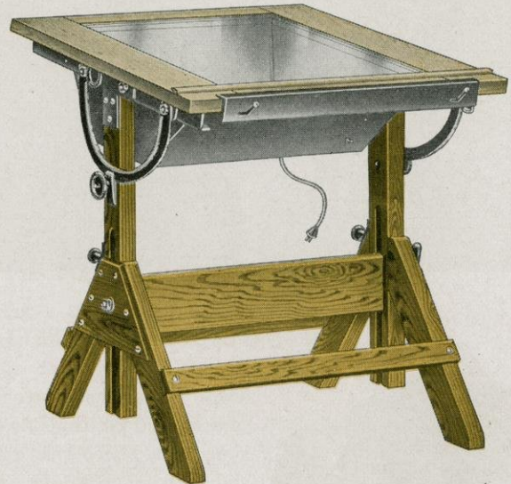
No. 183 FLUORESCENT TABLE —Equipped with two 15-watt, 18", T-8 Daylight Fluorescent Lamps for cool, even, glareless light. Ballast, starter and 10 feet of cord included. Plate glass center is 22 x 24", sandblasted on bottom side. Top overall is 31 x 32". Adjustable in slope and in height (32 \frac{3}{4} " x 42 \frac{1}{4} "). Entire top can slide forward or backward 15 \frac{1}{2} " on channel suspension. A roll of Scotch Tape is included. White enamel reflector pan, basswood top, hardwood frame. For 110-volt, 60-cycle alternating current only. Shipping Weight .....123 lbs.
