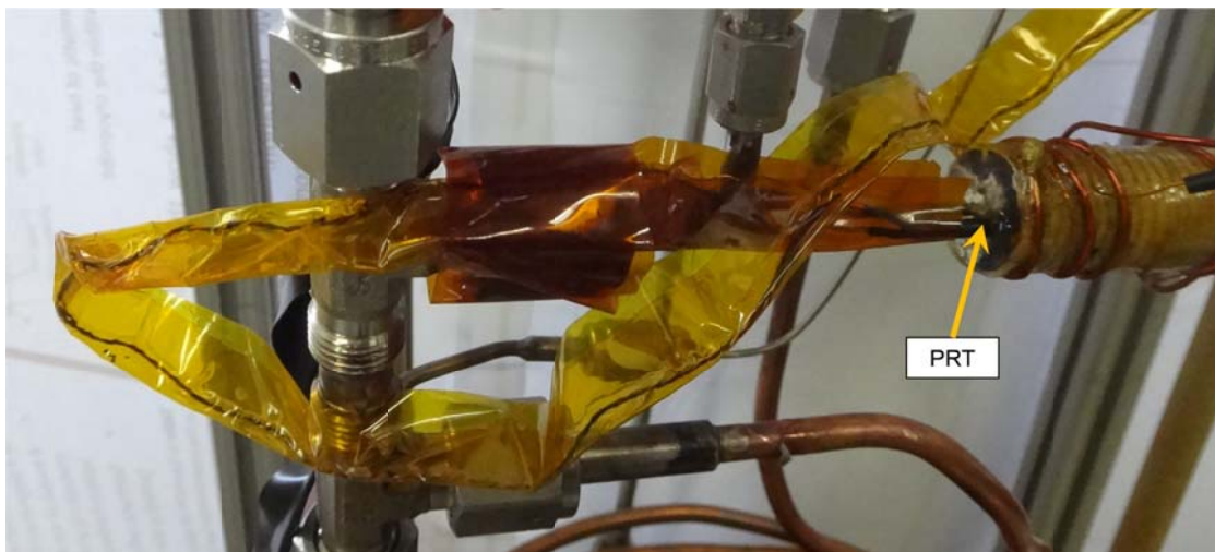
Figure 42. PRT installed in the copper block
