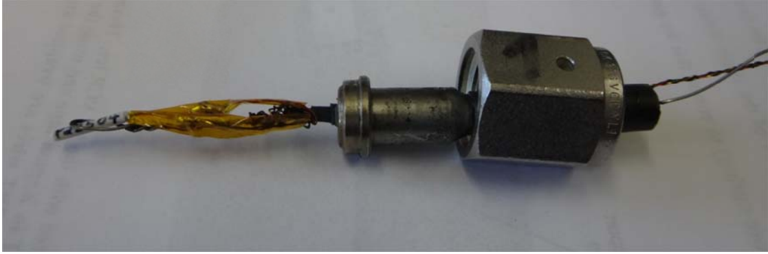
Figure 41. Temperature sensor designed to be immersed in the flow
