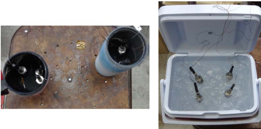
Figure 43. Calibration PRTs in liquid nitrogen (left side) and calibration PRTs in ice water bath (right side)
