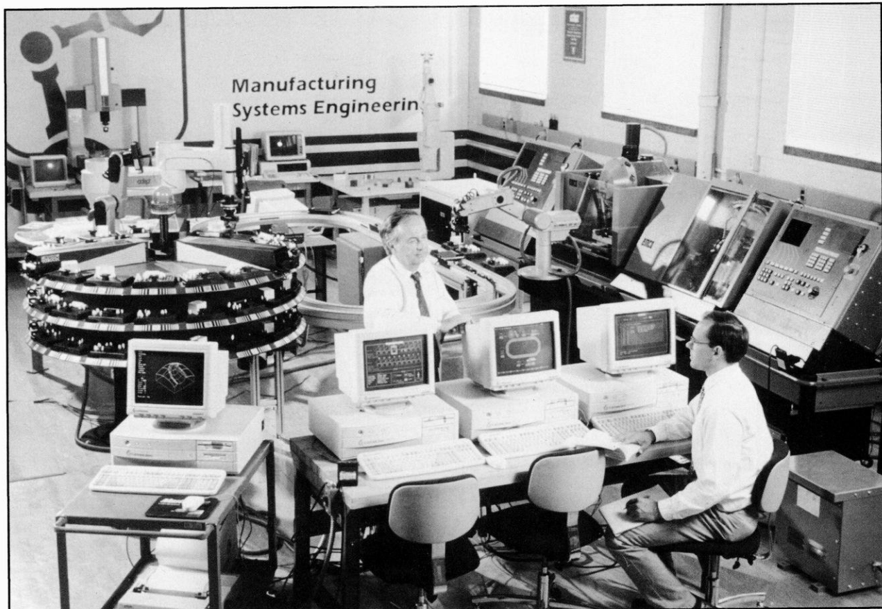
Industrial Engineering Professor Jerry Sanders looks on as MSE student Pat Galecki commands the IE/MSE Computer Integrated Manufacturing Cell from the master-cell controller.
