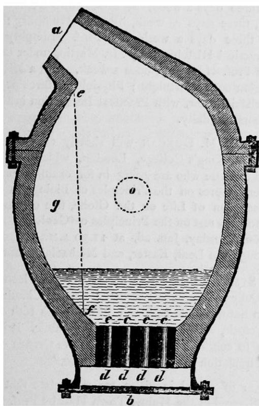
and all communicating with the space *d d*, into which opens the blast tube from a powerful blowing engine. The number of these blast holes varies from fifty or sixty to a hundred or more, according to the size of the converter.
