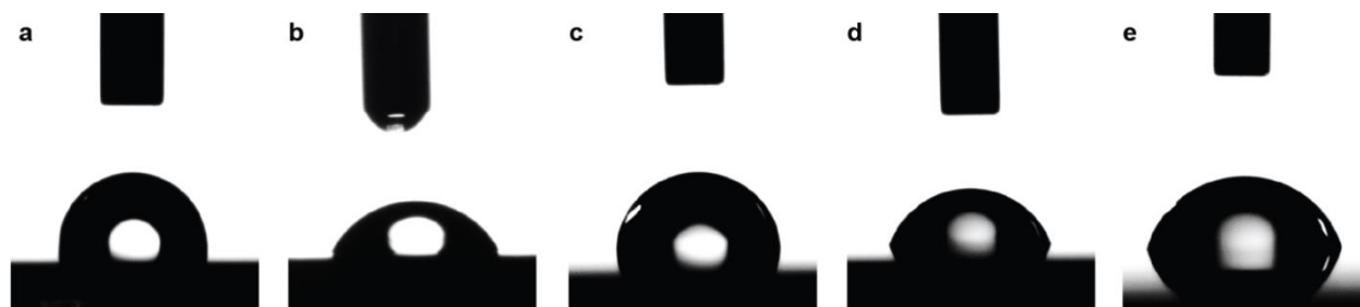
Figure 2.8 a-e, Water contact angles measurements of a graphene surface after solvent rinsing in chlorobenzene and toluene and annealing at 350 °C at \sim 10^{-5} torr for 2 h to remove residues and contamination introduced during processing (a), Ge(111) surface after O_2 (10 sccm) plasma etching at 50 W and 10 mtorr for 1-2 s (b), PS film (c), PMMA film (d), and PS-r-PMMA random brush neutral film consisting of 57% PS by weight composition (e).
