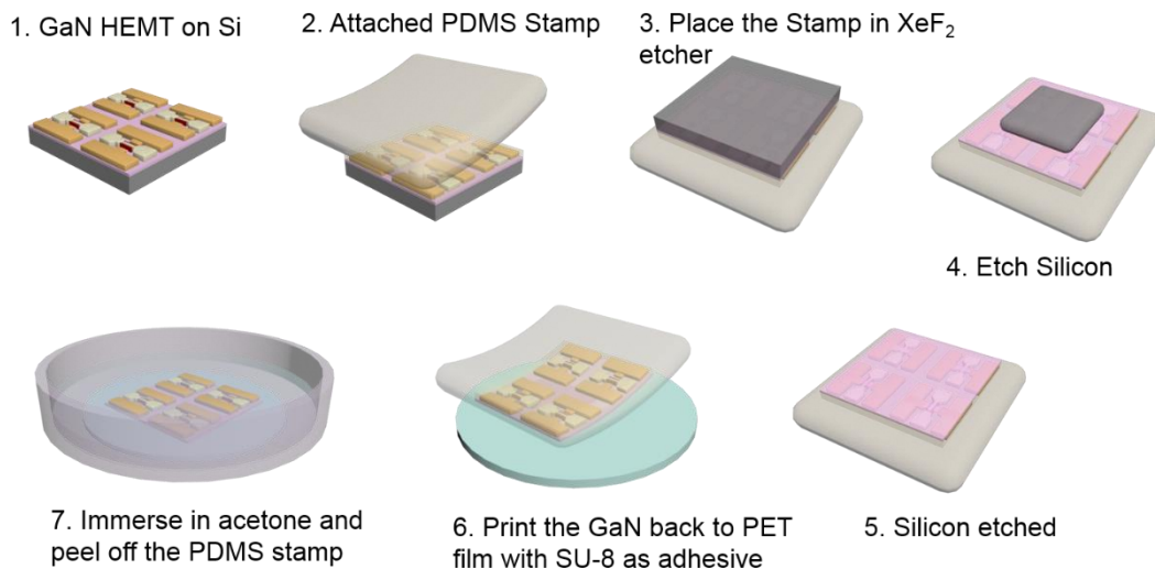
Figure 3.3 Process Flow of fabricating flexible GaN HEMT. The AlGaN/GaN thin film is transferred through PDMS stamp transferring and XeF 2 selective etching
