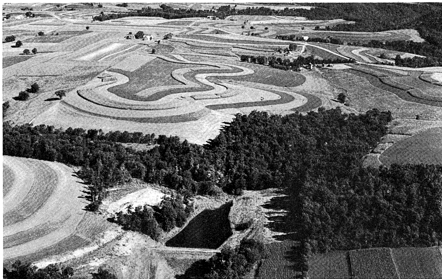
This 1963 photo of farms in the Coon Creek watershed shows the persistence of soil conserving practices introduced a quarter century earlier. Note water control structure and pond in the foreground and the contoured farm in background. (U.S.D.A. Soil Conservation Service, Madison Office)
