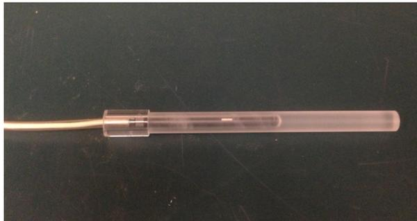
Figure 7.3: Photograph of the custom-designed PMMA cylindrical insert for A1SL ionization chamber.
