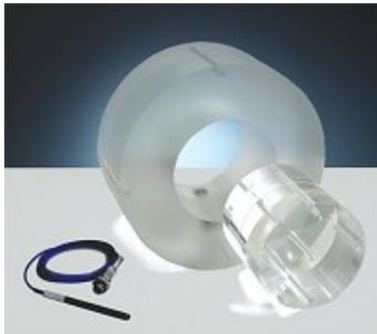
Figure 2.5: Photograph of the head and body CT dose phantoms and a pencil ionization chamber.
