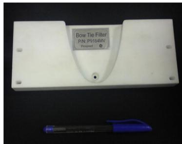
Figure 2.13: A photograph of a typical bowtie filter made of Teflon.
