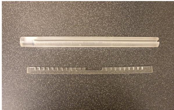
Figure 4.9: Photograph of the custom-designed TLD insert for  $z$ -direction profile measurements
