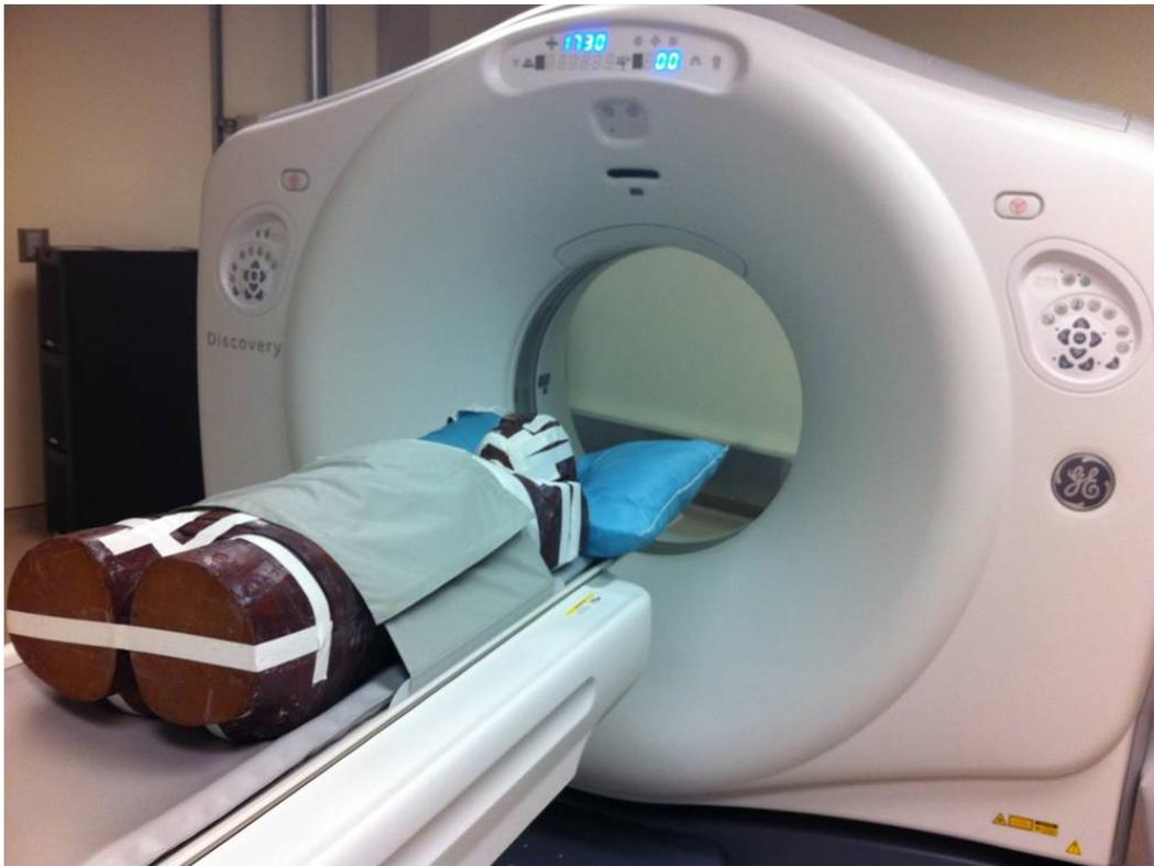
Figure 5.9: Photograph of the setup for the CT scan of a male anthropomorphic phantom.
