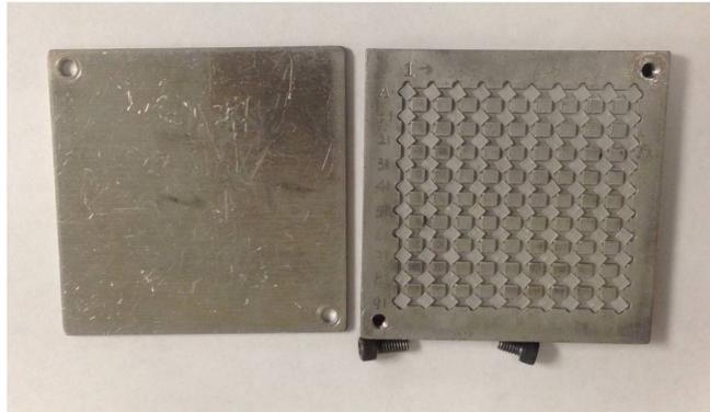
Figure 4.6: Photograph of an aluminum holder for TLD annealing.
