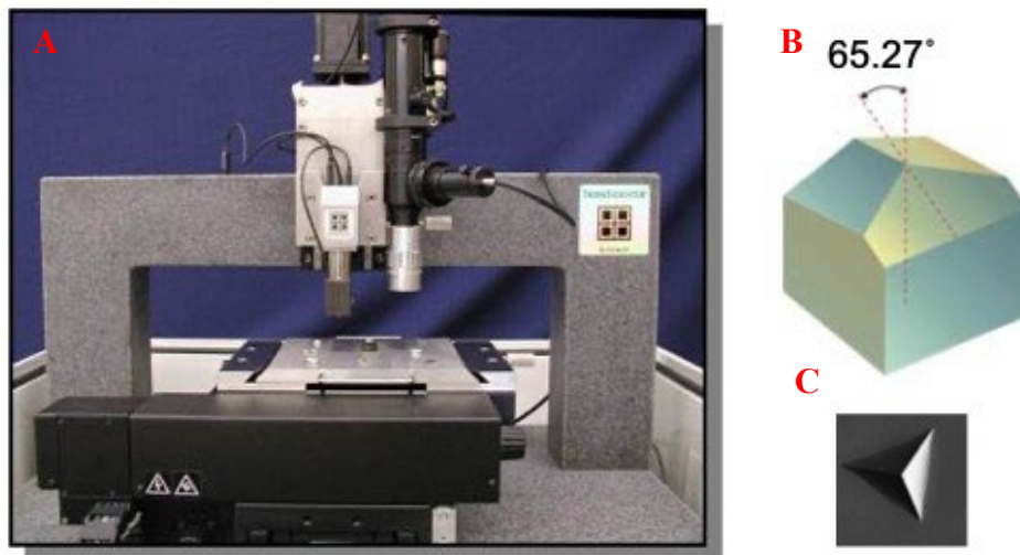
Figure 7 Ex situ nanoindentation test equipment illustration
