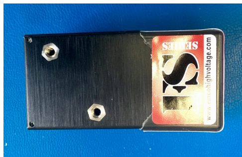
Figure 3.14, EMCO-FS40 High voltage power supply used for rotor excitation
